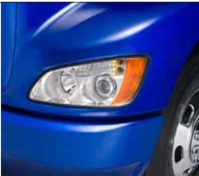
*An advanced halogen forward lighting system provides up to 30% more down-road coverage than conventional sealed beam designs.*
