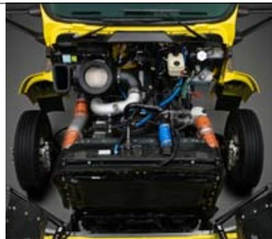
*The hood tilts a full 90 degrees for clear access to the engine compartment from both sides. All fluid level checks and fills can be handled quickly, standing in one place.*
